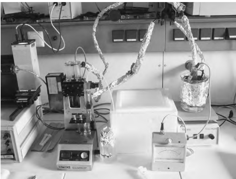
Figure 2 Water circulation at the stopped-flow apparatus. From left to right: electronics unit; sample-handling unit; ice container for cooling and hot plate for heating the circulating solution.
