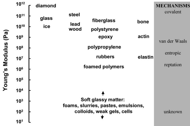
Fig. 2. The stiffness of common materials spans an exceedingly wide range, with living cells and other soft glasses at the lowest end of this range. Mechanisms accounting for matrix stiffness are shown at the right.
