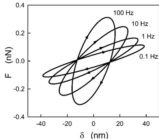
FIGURE 2 Fourier components at the oscillation frequency, corrected for the viscous drag, of force-indentation ( $F$ - $\delta$ ) loops measured at different frequencies at mean operating force  $F_o \sim 0.53 \text{ nN}$  and indentation depth  $\delta_o \sim 760 \text{ nm}$ . The loops became steeper and exhibited larger hysteresis as frequency increased. Data were obtained in the same cell as in Fig. 1.
