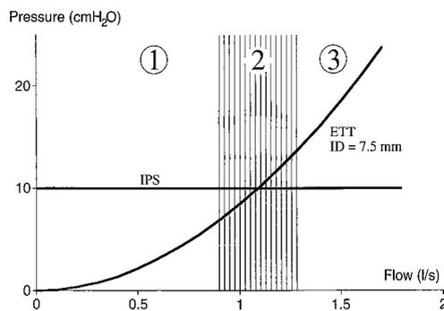
**Fig. 4** Inspiratory pressure/flow curve of an endotracheal tube (ETT) of 7.5 mm i.d. of original length (IPS inspiratory pressure support). See text for details
