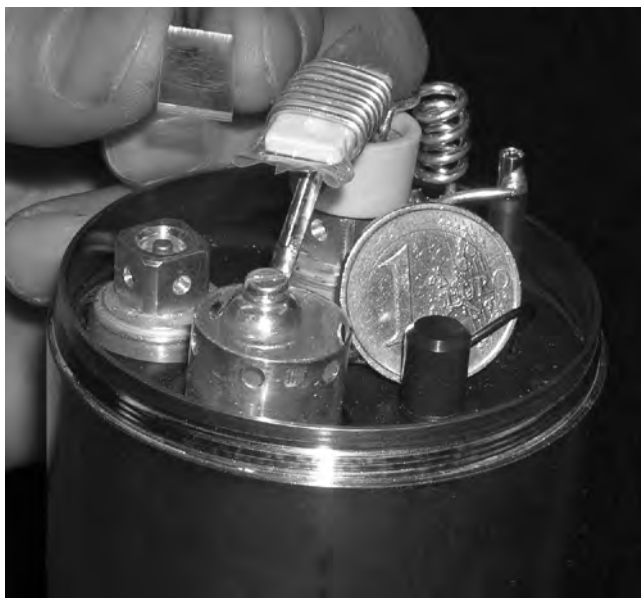
Figure 14 Solid-state NMR probe. The coils geometry has been adapted to the sample geometry. A stack of glass plates with several thousand lipid bilayers in between each pair is shown to the top left. The samples are protected and sealed before insertion into the flattened coil of the NMR probe. Before acquisition the NMR probe is introduced into the NMR magnet with the normal of the glass plates being oriented parallel to the magnetic field direction (Reproduced with permission).
