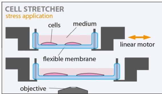
**Fig. 1.** Cell-stretcher. Cells are plated on an elastomeric PDMS-membrane coated with the extracellular matrix protein, fibronectin. The membrane is then stretched by a linear motor. The setup is attached to an inverted microscope to observe the cell behavior after stretch. All stretching experiments are carried out in an incubator at 37 °C, 5% CO<sub>2</sub>, 95% humidity at 20% stretch, 0.25 Hz and 1 h. The cartoon was kindly provided by Navid Bonakbar [32].
